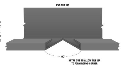
This clip on material should be cut to the required lengths, mitred at the corners, and the area where the flashing material and the rim of the bath meet, should be filled with a mould resistant Sanitory Grade sealant.
