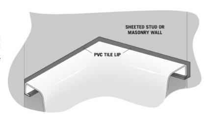
When the bath is installed, the minimum distance from the outside edge of the flange to the finished edge of the tiles shall be 10mm. The exposed area of the flange shall have continous fall to the inside of the bath.
